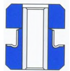
With steel reinforcement
